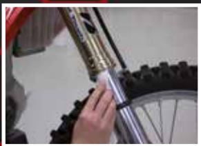
3. Clean space between the dust and oil seal
