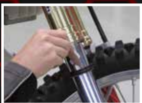
5. Apply grease on dust seal
