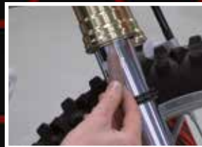
6. Apply grease between inner- and outertube
